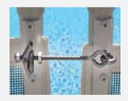
**Toggle Bolt Latches:** Made of a spring-actuated wing nut that passes through the eye of the opposing section. Once latched, no upward or downward motion can release it. To completely lock the latch, a jam nut can be threaded against the wing nut to prevent opening. Although they work well, they can loosen over time and have an industrial look.
